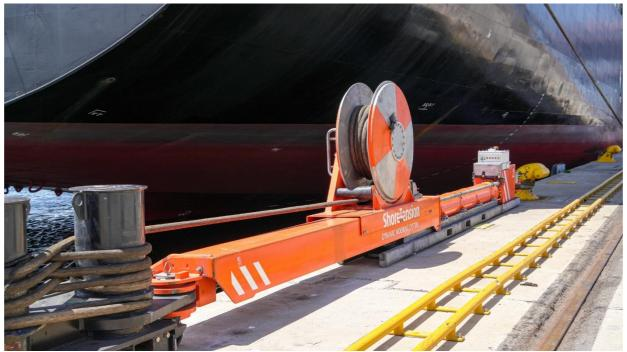
A hydraulic tension mooring unit is a system placed on the quayside to ensure the safety of docked vessels by mitigating the severity of long-wave effects on vessels.
